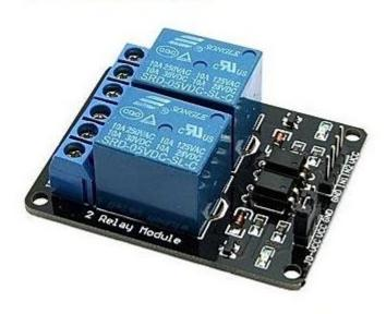
2 road with light coupling relay module
